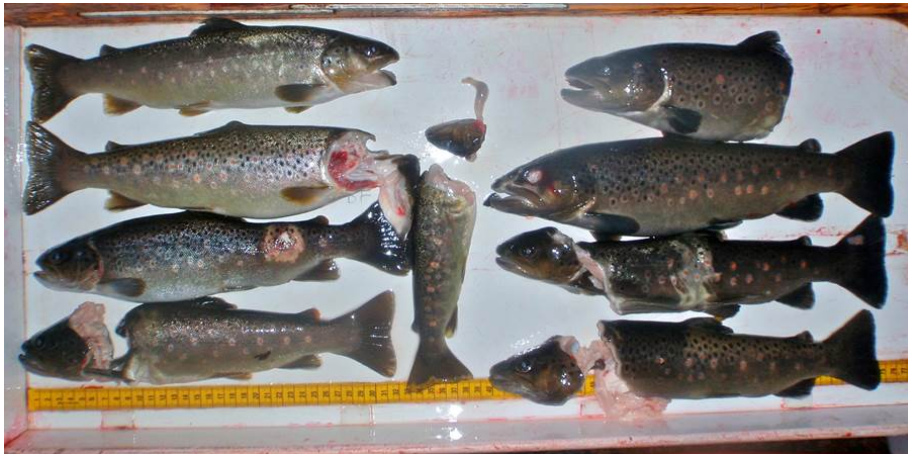
Figure 3: Salmonid injuries. Functional tests at the downstream fish movement structure at the hydroelectric plant Kostheim/mouth R. Main; December 2011. Source: BFS
